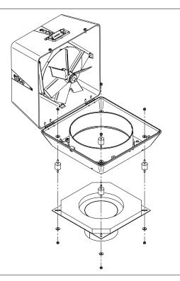
4 Fixate the flange to the chimney fan with the use of the vibration dampers supplied with the flange.
